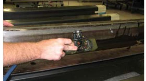
*Inspection of inner radius using equipment consisting of four single probes*
