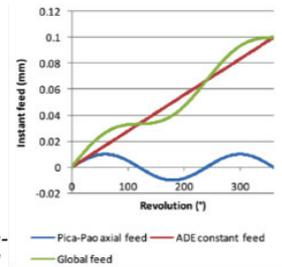
The diagram shows the variation in feed rate due to the generated vibration ("Pica-Pao").
