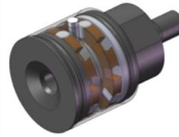
Principle of a tool holder with integrated bearing to create axial vibrations. 1,5 or 2,5 vibration cycles are generated per turn.
