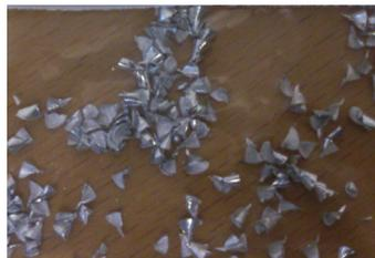
Generated extracted chips from vibration drilling in aluminium
