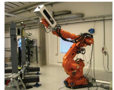
End-effector and robot used for testing robotic vibrating drilling
