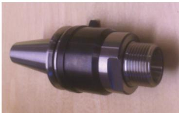
The ISO 25 tool holder with bearing for vibration drilling
