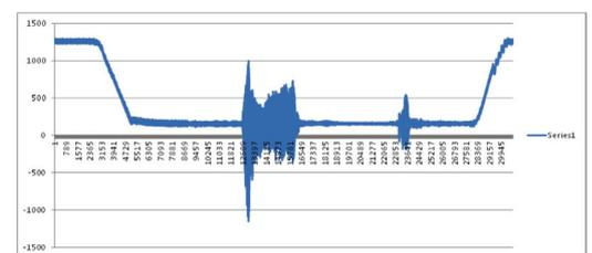
Measured axial cutting (reacting) forces in newton (Y) created on the end-effector during one drilling & countersink cycle
