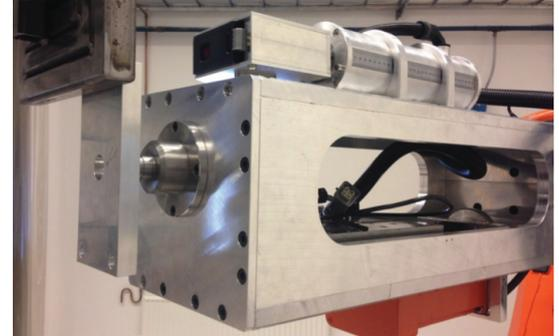
*Robotic drilling with X-laser installed on top of end-effector.*
