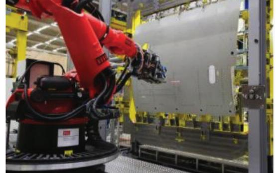
Robotic drilling without force sensing at Saab Aerostructure
