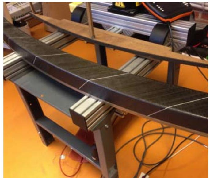
*Formed 45/-45 degree pair with reference for fibre angle measurement.*
