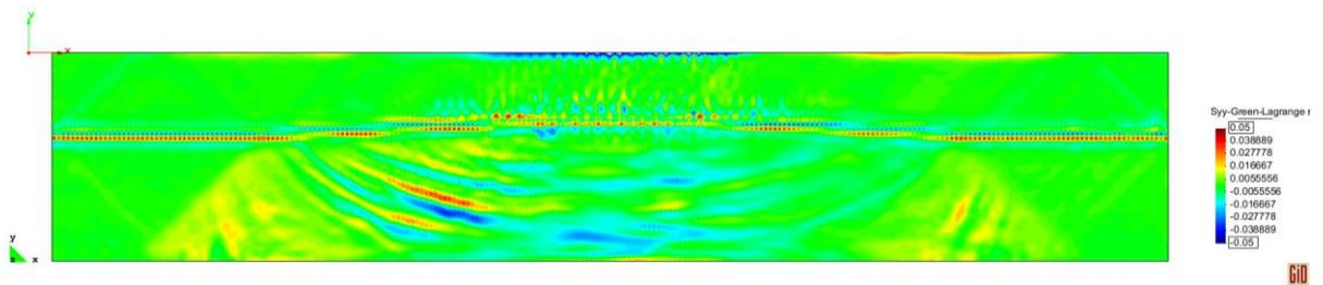
Figure 7b: Compression in terms of  $S_{yy}$  in the joggle area of layer 3 [0] in the reference spar with quasi-isotropic lay-up.
