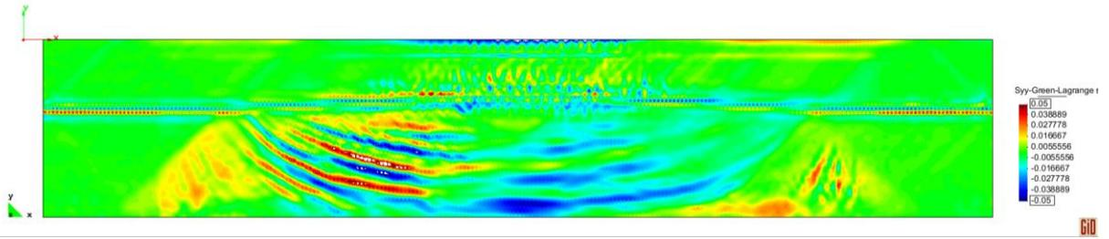
Figure 7a: Compression in terms of  $S_{yy}$  in the joggle area of layer 3 [0] in the spar with quasi-isotropic lay-up with added contact surfaces in the [-45] / [0] interlayers.
