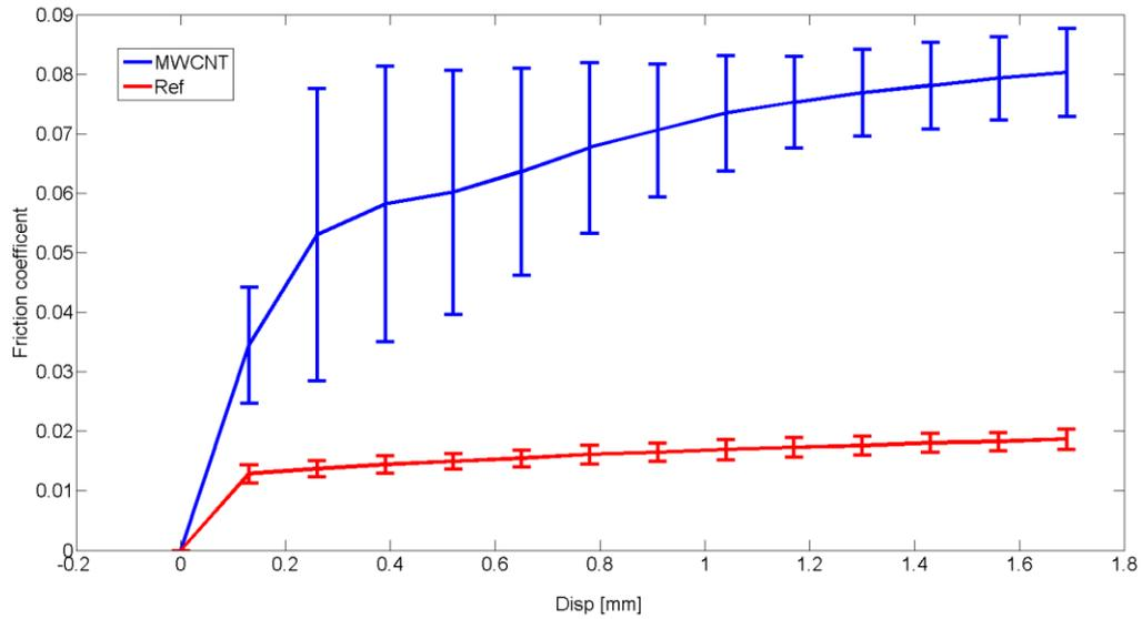
Figure 5b: Interply friction measurement graphs.
