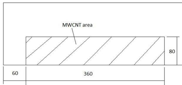
Figure 1 MWCNT area orientation in flat lay-up before HDF.
