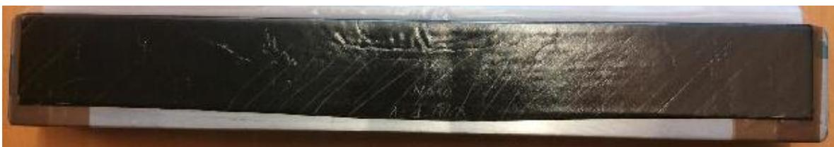
Figure 6: Out-of-plane wrinkling in the joggled area of a spar with a kvasi-isotropic lay-up with MWCNTs in the [-45] / [0] interlayers.
