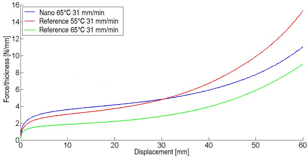
Figure 5a: Resulting load curves from intraply shear test.
